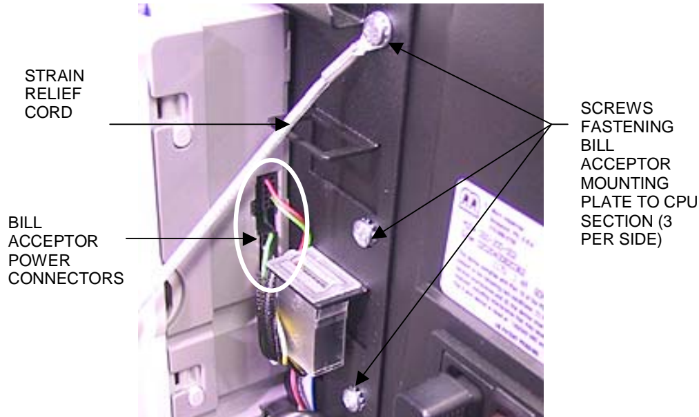
FIGURE 2 - REAR VIEW OF BILL ACCEPTOR MOUNTING PLATE
