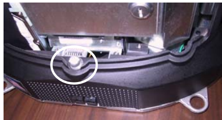
FIGURE 2 - SCREW IN CENTER OF BOTTOM COVER
