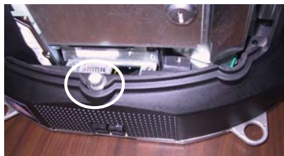
FIGURE 2 - SCREW IN CENTER OF BOTTOM COVER
