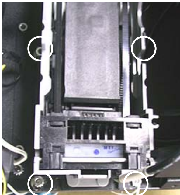
FIGURE 4 - SCREWS SECURING BILLACCEPTOR TO MOUNTING PLATE
