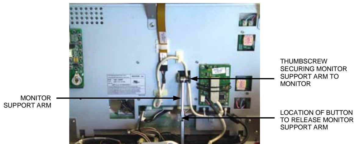
FIGURE 2 - SUPPORT ARM CONNECTION TO MONITOR
