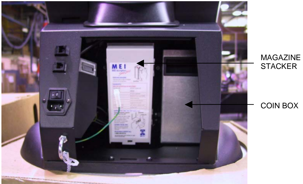
FIGURE 1 - ELITE EDGE - BILL ACCEPTOR ACCESS/REMOVAL
