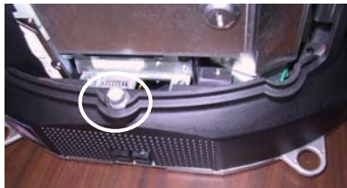
FIGURE 2 - SCREW IN CENTER OF BOTTOM COVER
