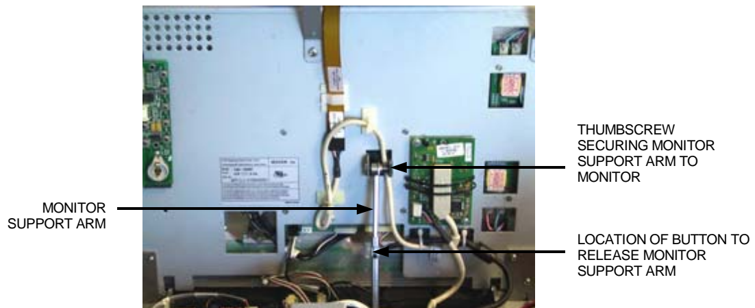
FIGURE 2 - REAR VIEW OF MONITOR ASSEMBLY
