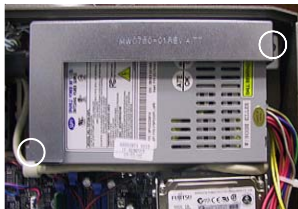
FIGURE 2 - POWER SUPPLY MOUNTING SCREWS (2 PLACES)
